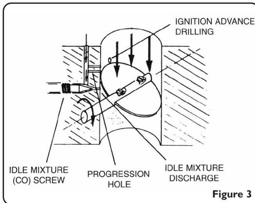
In such carburettors, idle speed can be of the adjustable throttle stop type (Figure 3-7)
